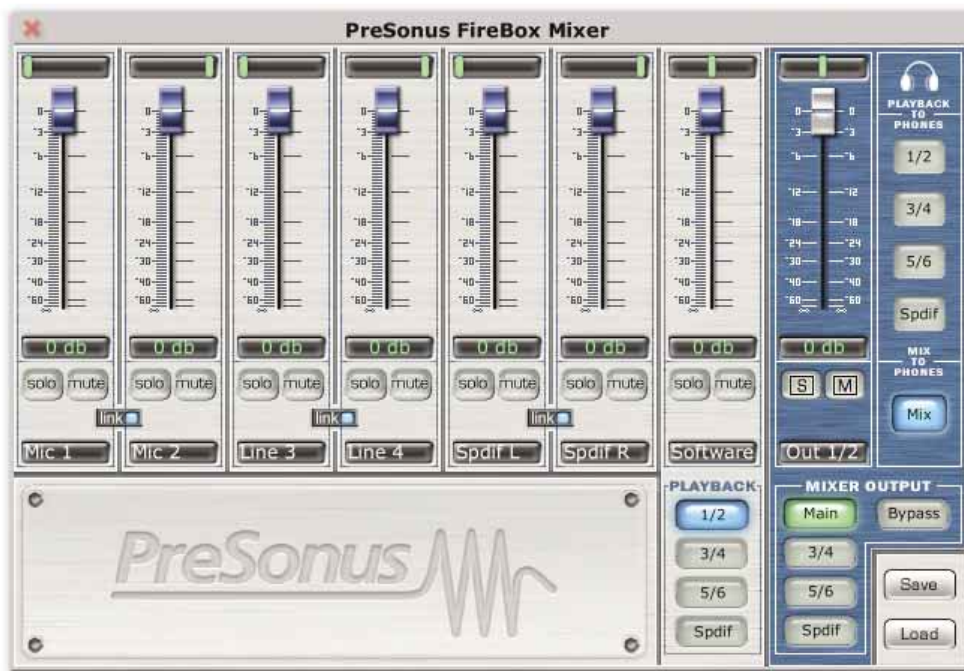
The Firebox Mixer application, as it appears on the Mac — the PC version is graphically identical. Looks great, and easy to understand. With input monitoring disabled on your host audio application, this is how the Mixer would look for zero-latency monitoring.
